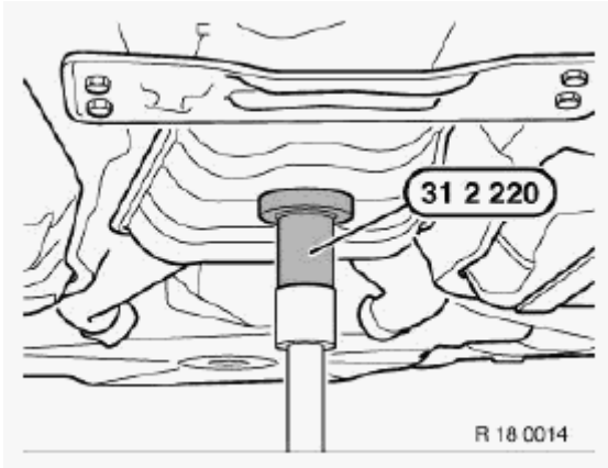
Fig. 40: Supporting Exhaust System Using Special Tool 31 2 220 Courtesy of BMW OF NORTH AMERICA, INC.
