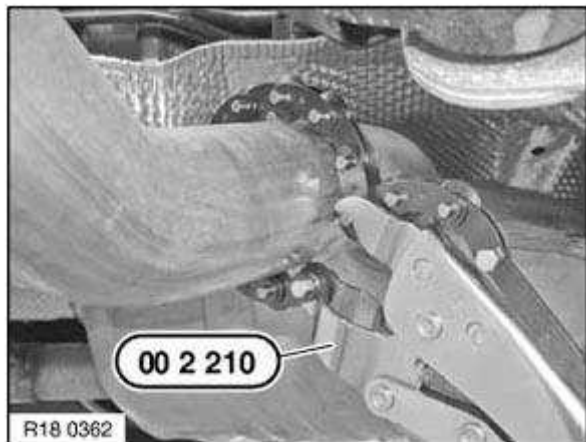
Fig. 46: Cutting Exhaust Pipe Using Special Tool 00 2 210 Courtesy of BMW OF NORTH AMERICA, INC.
