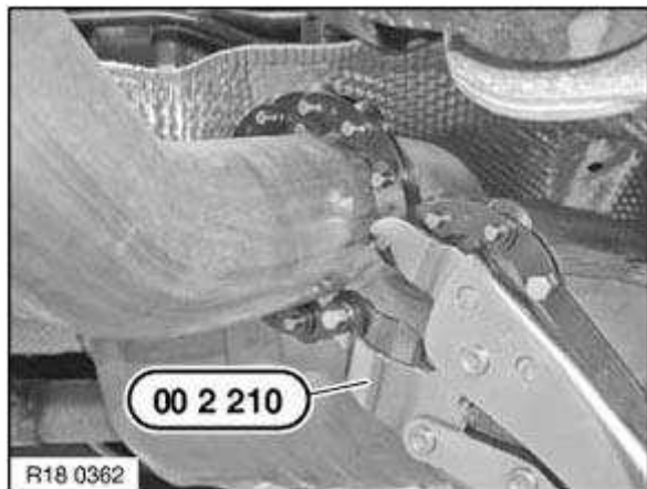
Fig. 34: Cutting Exhaust Pipe Using Special Tool 00 2 210 Courtesy of BMW OF NORTH AMERICA, INC.
