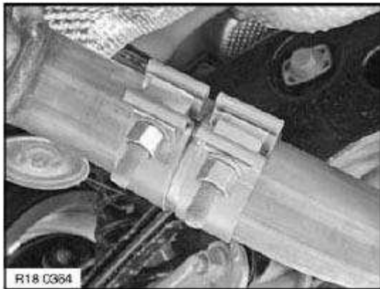
Fig. 54: Connecting Center Muffler To Rear Muffler Using Clamp Courtesy of BMW OF NORTH AMERICA, INC.
