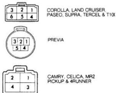
Fig. 1: Front Wiper Motor Terminal ID Courtesy of Toyota Motor Sales, U.S.A., Inc.
