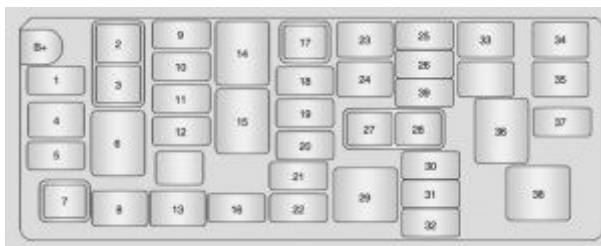
Chevrolet Spark – fuse box – engine compartment
