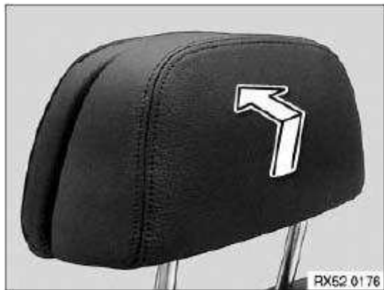
Fig. 46: Clipping Cover Onto Carrier Section Courtesy of BMW OF NORTH AMERICA, INC.
