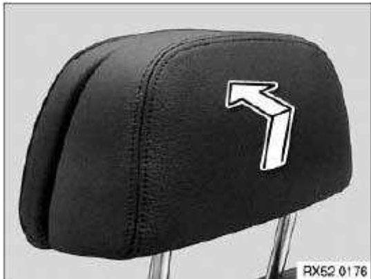
Fig. 141: Clipping Cover Onto Carrier Section Courtesy of BMW OF NORTH AMERICA, INC.
