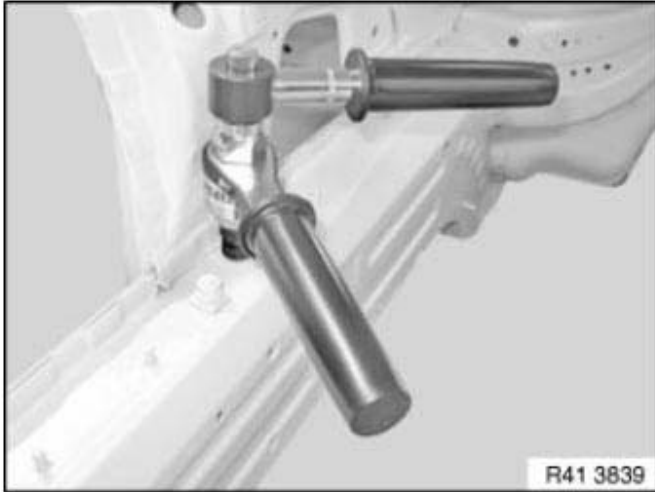
Fig. 6: Setting Rivet Nut With Hand Rivet Gun Courtesy of BMW OF NORTH AMERICA, INC.
