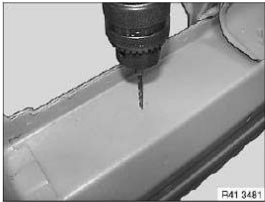
Fig. 2: Drilling Bore Using Drill Bit Courtesy of BMW OF NORTH AMERICA, INC.
