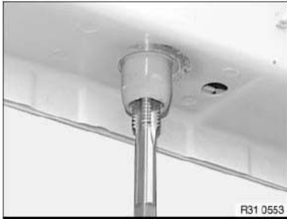
Fig. 7: Inserting Helicoil Thread On Locating Thread Courtesy of BMW OF NORTH AMERICA, INC.
