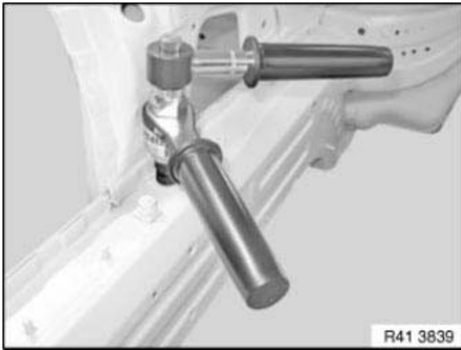
Fig. 23: Setting Rivet Nut With Hand Rivet Gun Courtesy of BMW OF NORTH AMERICA, INC.
