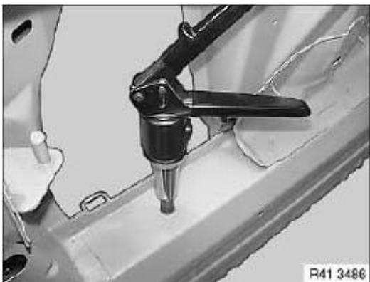
Fig. 22: Setting Rivet Using With Hand Rivet Gun
