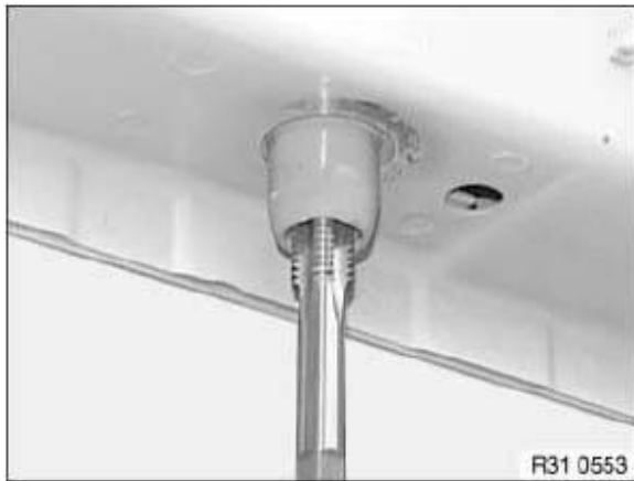
Fig. 12: Inserting Helicoil Thread On Locating Thread Courtesy of BMW OF NORTH AMERICA, INC.
