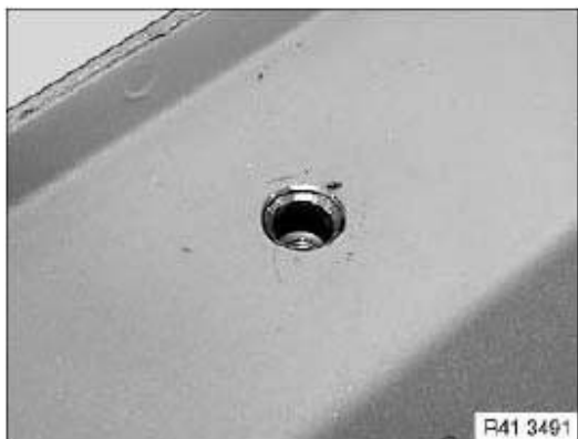
Fig. 18: Identifying Cavity Of Rivet Shank Courtesy of BMW OF NORTH AMERICA, INC.
