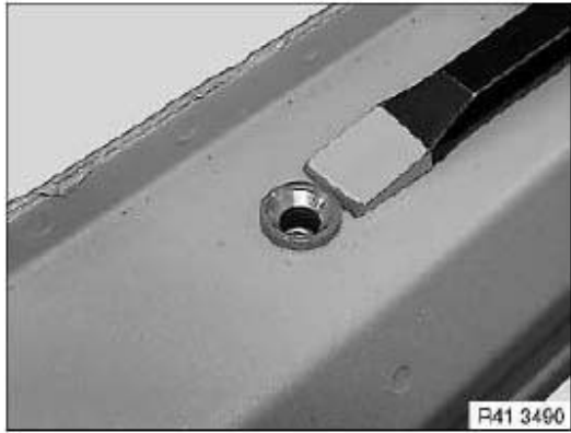
Fig. 17: Knocking Rivet Head Using Chisel Courtesy of BMW OF NORTH AMERICA, INC.
