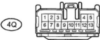
Fig. 46: Identifying 4Q Main Body ECU Connector Terminals Courtesy of TOYOTA MOTOR SALES, U.S.A., INC.
