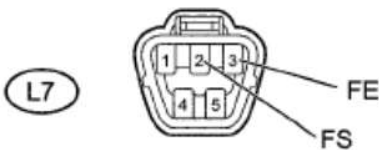
Fig. 41: Identifying F2 Combination Meter Assembly Connector Terminals Courtesy of TOYOTA MOTOR SALES, U.S.A., INC.
