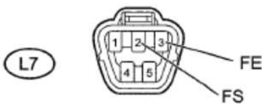
Fig. 30: Identifving F2 Combination Meter Assembly Connector Terminals
