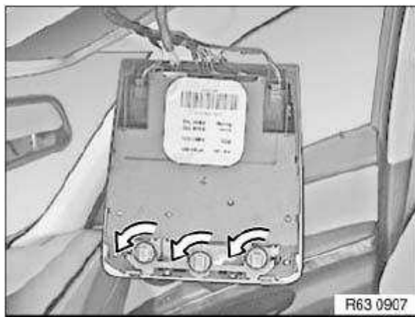
Fig. 60: Turning Bulb Holder Courtesy of BMW OF NORTH AMERICA, INC.
