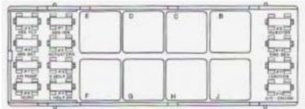
Pontiac Firebird – fuse box – engine compartment
