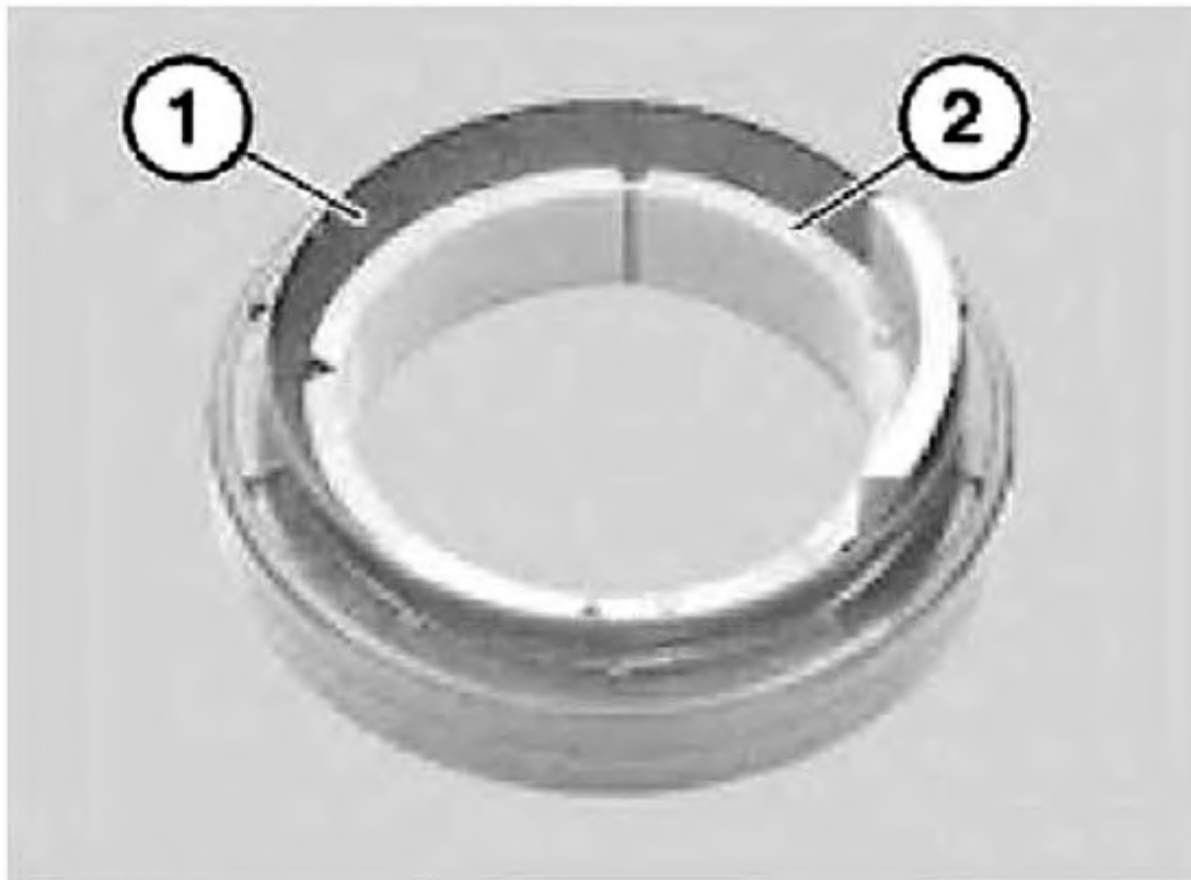
Fig. 16: Removing Protective Sleeve
