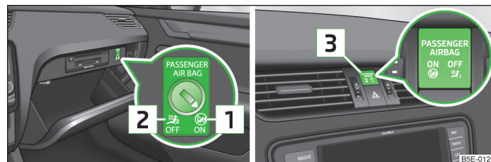
Fig. 170 Key-operated switch for the front passenger airbag/warning light for front seat passenger airbag deactivation
