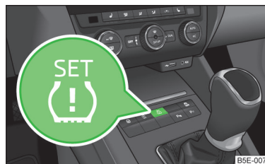
Fig. 191 Button for setting the tyre inflation pressure control value
