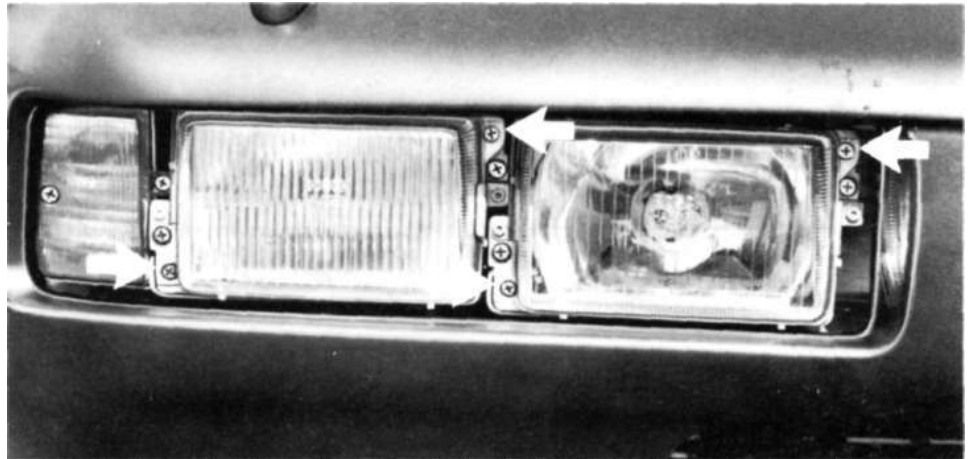
Upper adjustment screw = lateral adjustment Lower adjustment screw = vertical adjustment
