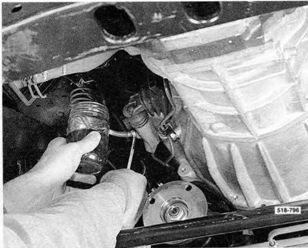
Bleeding the clutch hydraulic system.
