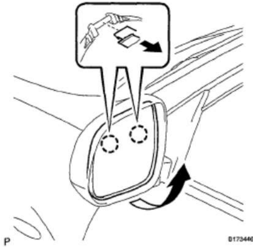
Fig. 29: Removing Outer Mirror Glass
