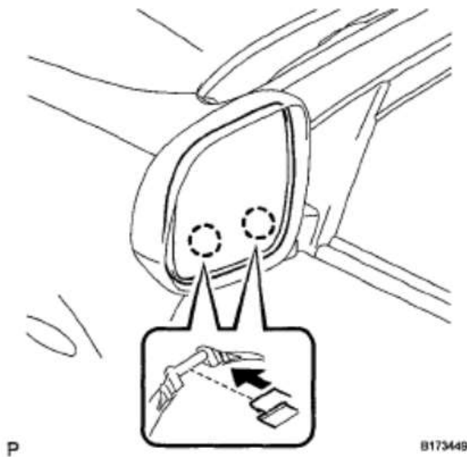
Fig. 35: Engaging Claws On Lower Part Of Outer Mirror Glass To Outer Mirror Courtesy of TOYOTA MOTOR SALES, U.S.A., INC.
