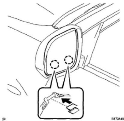
Fig. 37: Engaging Claws On Lower Part Of Outer Mirror Glass To Outer Mirror Courtesy of TOYOTA MOTOR SALES, U.S.A., INC.
