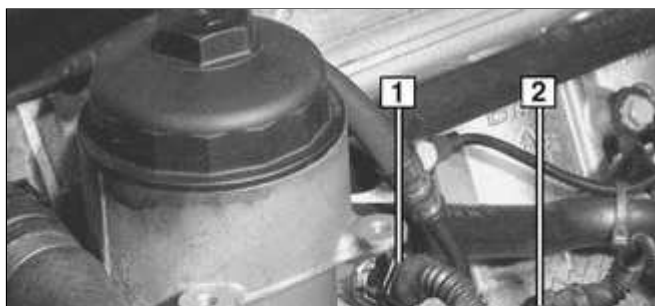
Fig. 26 Left front of engine, at oil filter housing 1 - Oil/coolant temperature sensor 2 - Oil pressure switch
