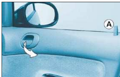
Opening the doors from inside
