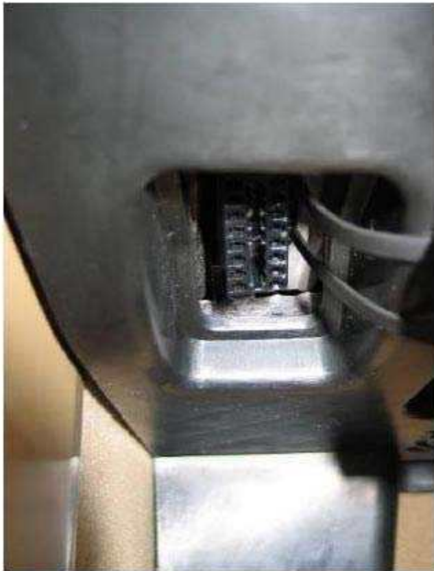
Fig. 30: Identifying DLC And Removed Cover Location Courtesy of BMW OF NORTH AMERICA, INC.
