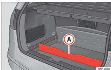
Fig. 110 Boot floor partition.
