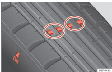
Fig. 152 Tyre tread wear indicators.
