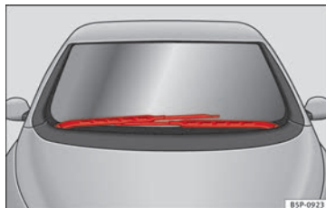
Fig. 169 Windscreen wipers in the service position.
