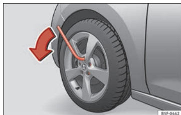
Fig. 157 Changing a wheel: loosen the wheel bolts.
