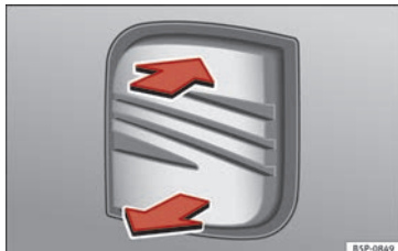
Fig. 53 Rear lid: opening from the outside.
