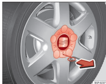
Fig. 155 Changing a wheel: remove the wheel trim.
