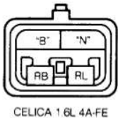
Fig. 4: Park/Neutral Switch Terminal ID (1.6L) Courtesy of Toyota Motor Sales, U.S.A., Inc.
