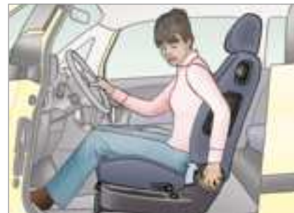
3. Seat back angle adjustment.
