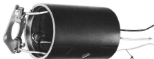
A = newly soldered earth line
