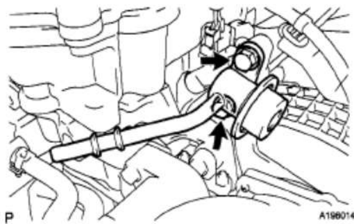
Fig. 69: Locating Fuel Pressure Pulsation Damper Bolts Courtesy of TOYOTA MOTOR SALES, U.S.A., INC.
