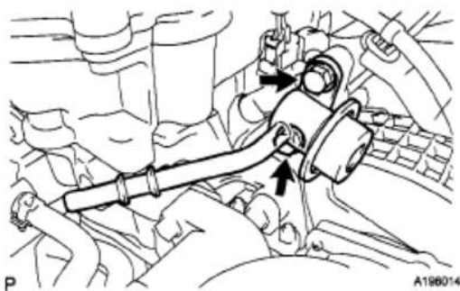
Fig. 67: Locating Fuel Pressure Pulsation Damper Bolts Courtesy of TOYOTA MOTOR SALES, U.S.A., INC.
