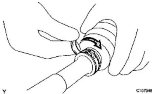
Fig. 36: Installing Front Axle Outboard Joint Boot Clamp LH Onto Outboard Joint Boot Courtesy of TOYOTA MOTOR SALES, U.S.A., INC.
