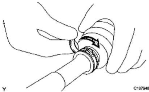
Fig. 47: Installing Front Axle Outboard Joint Boot Clamp LH Onto Outboard Joint Boot Courtesy of TOYOTA MOTOR SALES, U.S.A., INC.
