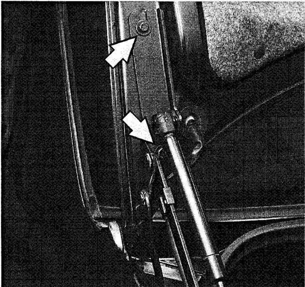
Fig. 2. Trunk lid hinge bolts (arrows). Loosen upper bolt and remove lower bolt.
