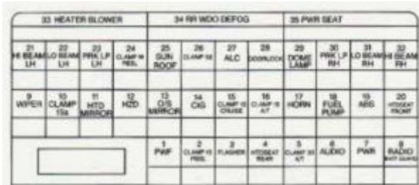
Cadillac Catera – fuse box diagram – instrument panel
