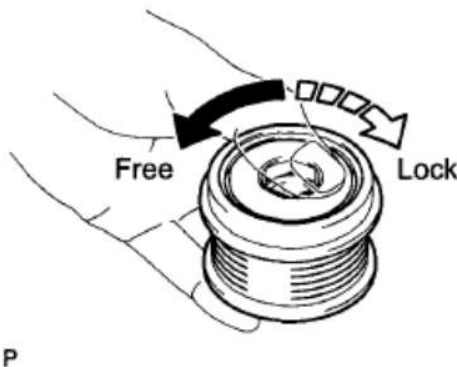
Fig. 32: Inspecting Generator Pulley With Clutch Courtesy of TOYOTA MOTOR SALES, U.S.A., INC.
