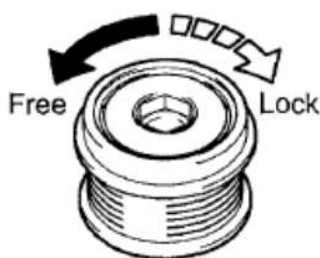
Fig. 9: Checking Lock Function Of Clutch Pulley Courtesy of TOYOTA MOTOR SALES, U.S.A., INC.
