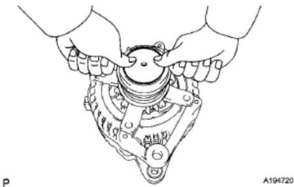
Fig. 43: Installing Generator Pulley Cap To Pulley
