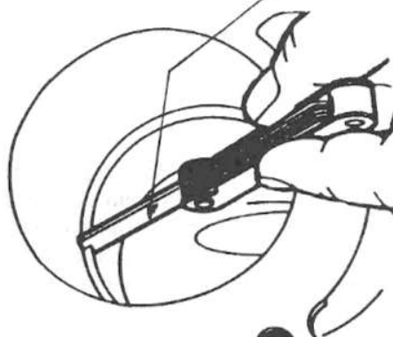
Measuring piston ring end gap Feeler gauge
