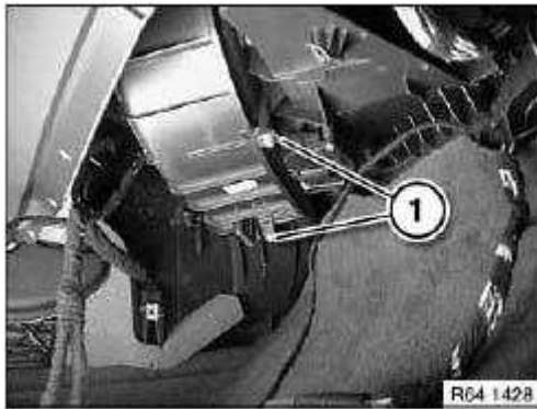
Fig. 15: Identifying Air Duct Screw Location Courtesy of BMW OF NORTH AMERICA, INC.
