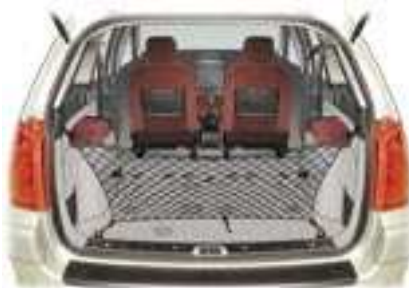
Luggage retaining net, "hammock" version at the roller
