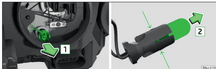
Fig. 187 Change the light bulb for the parking light
