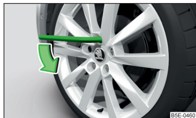
Fig. 161 Changing a wheel: Loosening the wheel bolts
