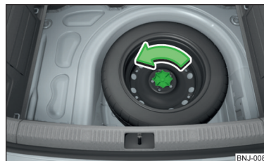
Fig. 159 Taking the wheel out
