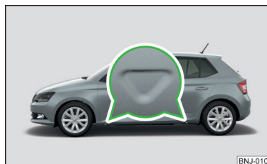
Fig. 162 Jacking points for positioning lifting jack
