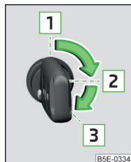
Fig. 105 Positions of the vehicle key in the ignition lock
