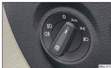
Fig. 43 Light switch: AUTO position
