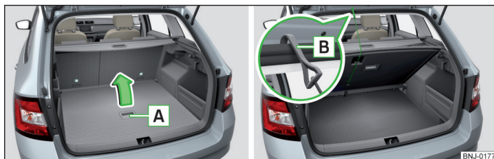
Fig. 94 Fold up variable loading floor / secure variable loading floor
