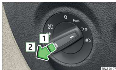
Fig. 44 Light switch: Turn on front and rear fog light
