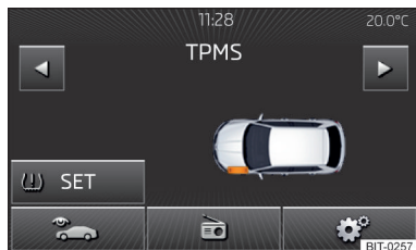
Fig. 127 Key for storing the pressure values / example of the display: the system indicates a pressure change in the front left tyre
