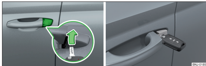
Fig. 172 Handle on the driver's door: covered locking cylinder / locking cylinder with key
