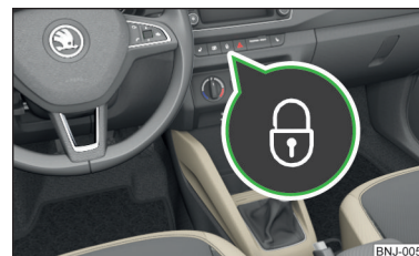
Fig. 34 Central locking button
