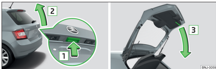
Fig. 37 Opening / closing tailgate
