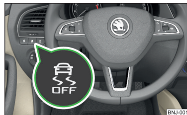
Fig. 113 System button: Activating/deactivating TCS
