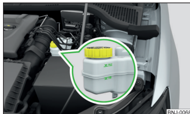
Fig. 149 Brake fluid reservoir
