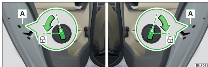
Fig. 173 Emergency locking: Left/right rear door
