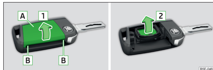
Fig. 171 Remove cover/take out battery
