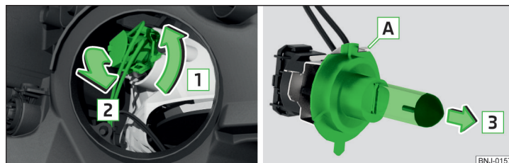
Fig. 189 Changing the bulb for the low beam
