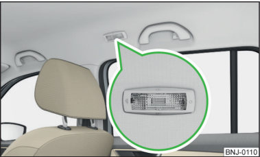
Fig. 47 Interior lights at the rear
