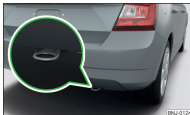
Fig. 170 Rear towing eye
