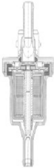
Sectional view of canister control valve
