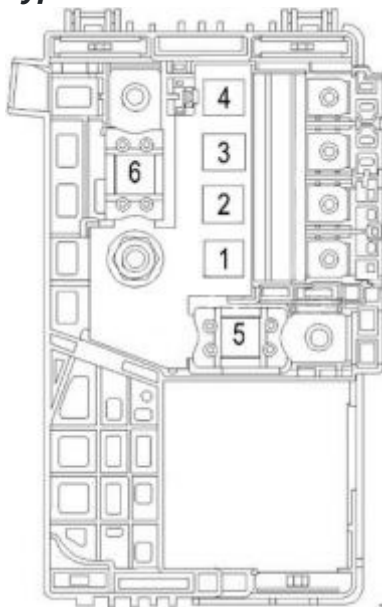
Chevrolet Malibu – fuse box diagram – fusible link block type 1
