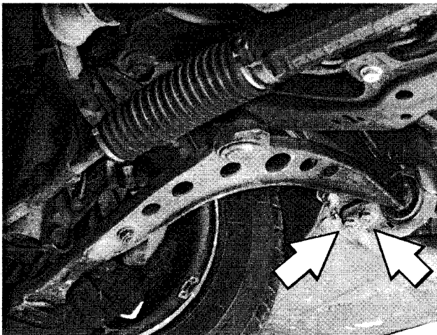
Fig. 9. Control arm bushing carrier bolts (arrows).
