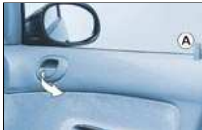
Opening the doors from inside*
