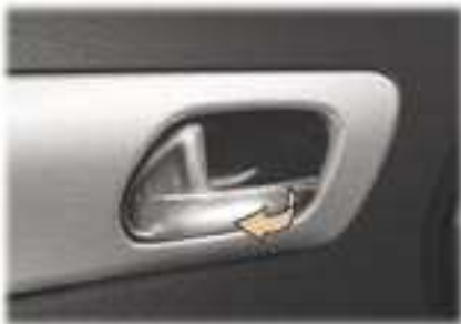
Opening the doors from inside
