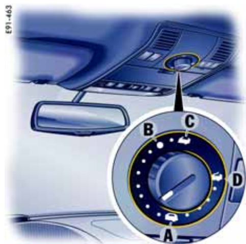
Switch in the roof console
