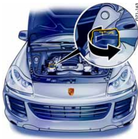
Engine oil filling point on Cayenne S, Cayenne GTS, Cayenne S Transsyberia
