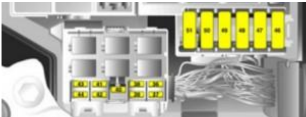
Vauxhall Tigra – fuse box – engine compartment – others engine
