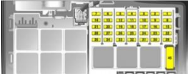
Vauxhall Tigra – fuse box – engine compartment -engine z13dt
