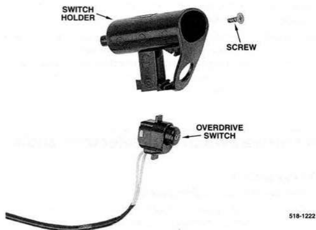
Overdrive switch components removed from the handle.
