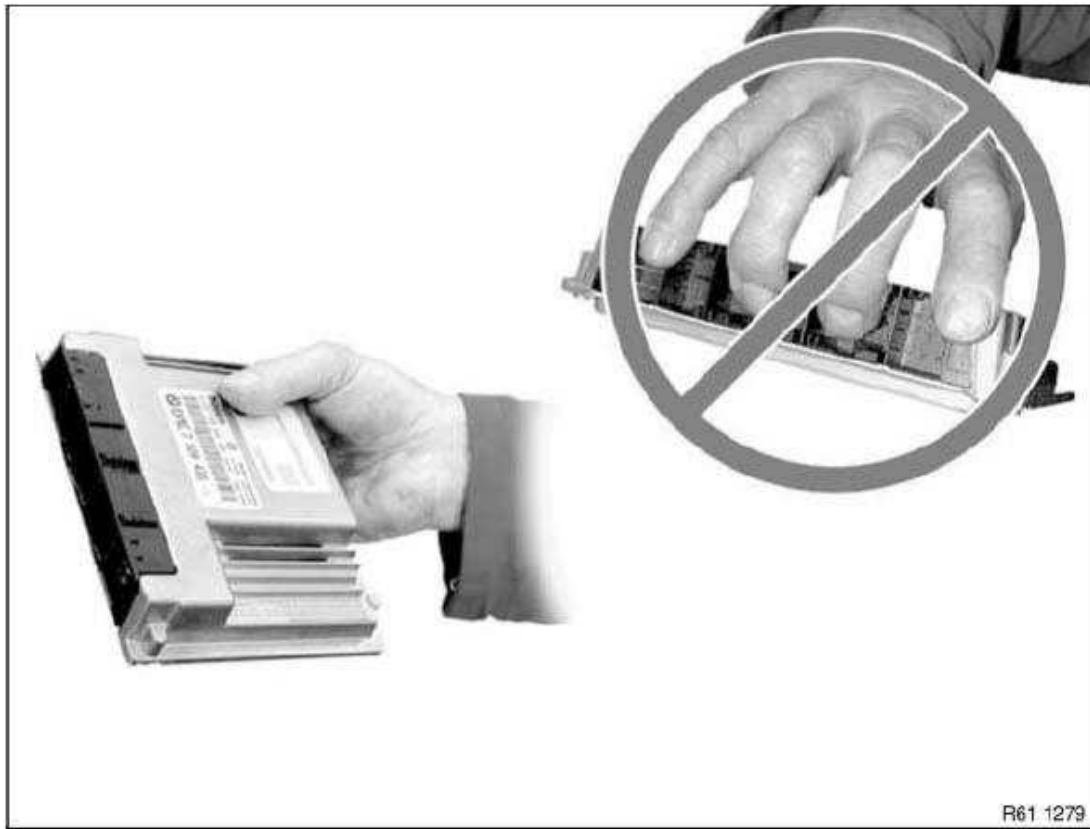
Fig. 234: Precaution For Mechatronic Control Unit Courtesy of BMW OF NORTH AMERICA, INC.
