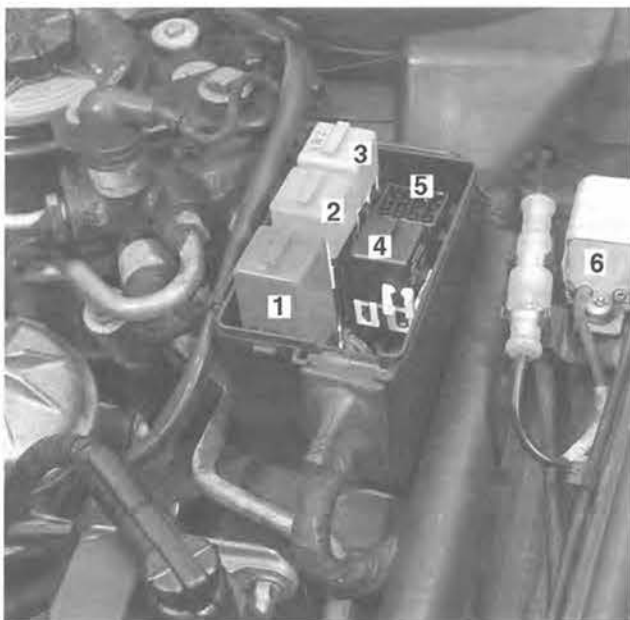
610-8 Auxiliary relay panel I
