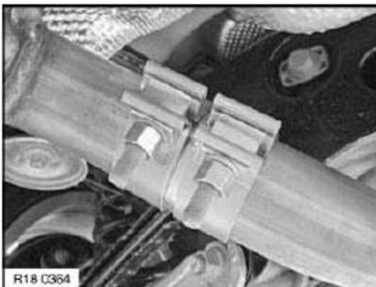
Fig. 13: Tightening Centre Clamps
