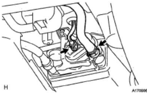
Fig. 21: Locating Hose And Connector Courtesy of TOYOTA MOTOR SALES, U.S.A., INC.
