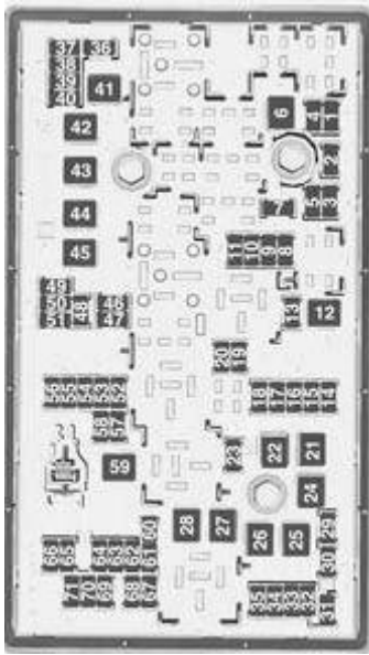
Vauxhall Insignia – fuse box – engine compartment
