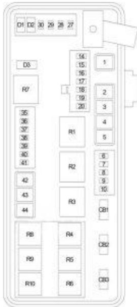
Dodge Magnum – fuse box diagram – luggage compartment
