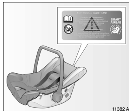
Vauxhall safety cradle with transponders From birth up to a weight of 10 kg. The transponders are integrated in the seat cushion.
