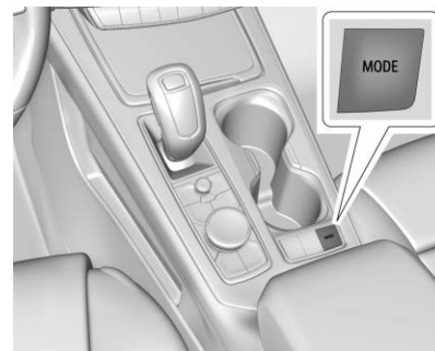
Driver Mode Control Switch
