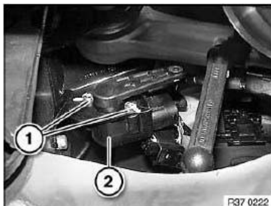
Fig. 66: Identifying Ride-Height Sensor And Screws Courtesy of BMW OF NORTH AMERICA, INC.
