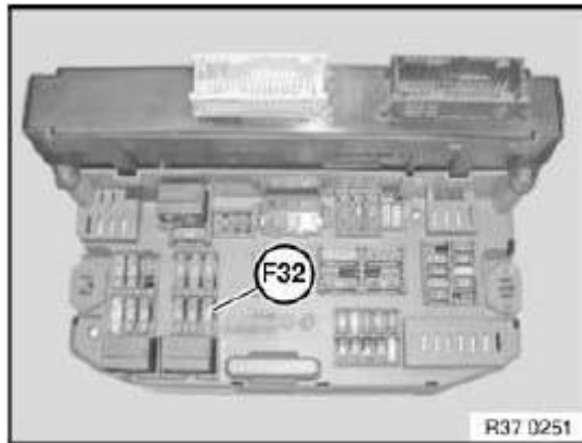
Fig. 7: Identifying Fuse (F32)
