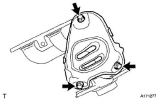
Fig. 9: Locating No. 2 Exhaust Manifold Heat Insulator Bolts Courtesy of TOYOTA MOTOR SALES, U.S.A., INC.
