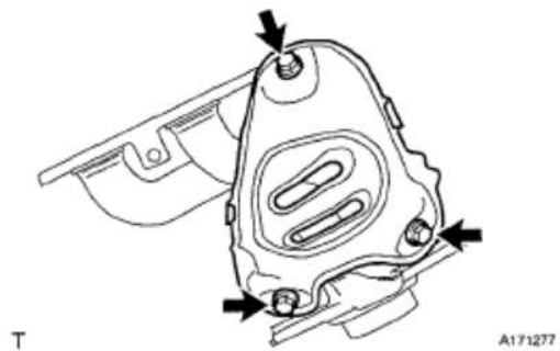
Fig. 8: Locating No. 2 Exhaust Manifold Heat Insulator Bolts
