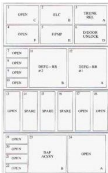
Oldsmobile Aurora – fuse box – rear compartment driver side fuse block
