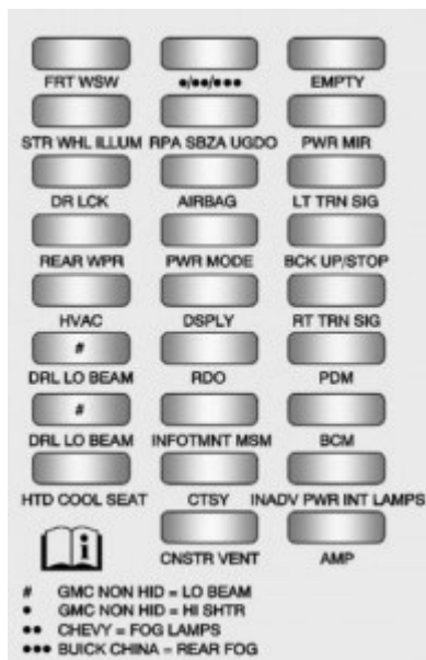
Buick Enclave 2013 – fuse box – instrument panel block
