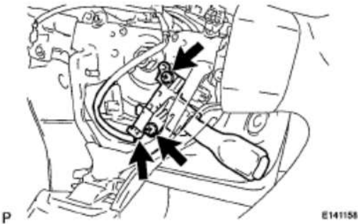
Fig. 30: Identifying Cruise Control Main Switch Screws Courtesy of TOYOTA MOTOR SALES, U.S.A., INC.
